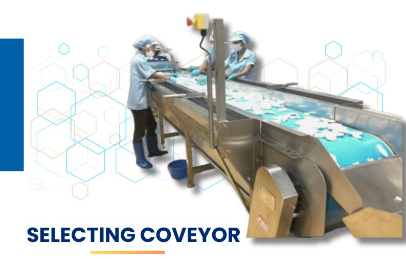
This conveyor is designed to transport and sort coconuts based on size, quality, or other criteria. It uses a conveyor belt system to move coconuts along a path where they are inspected and sorted, ensuring only the desired coconuts proceed to the next stage of processing.
